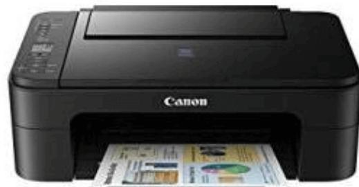
The inkjet printer is a non-impact printer that prints images and characters by spraying fine, ionized drops of ink. The print head has tiny nozzles to spray the ink. The printer head moves back and forth and sprays ionized drops of ink on the paper, which is fed through the printer. These drops pass through an electric field that guides the ink onto the paper to print correct images and characters.
