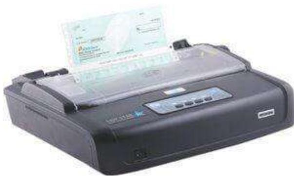
Dot Matrix Printer is an impact printer. The characters and images printed by it are the patterns of dots. These patterns are produced by striking the ink soaked ribbon against the paper with a print head. The print head
