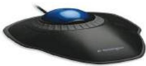
It is a stationary input device that has ball mechanism to move the pointer or cursor on the screen. The ball is half inserted in the device and can be easily rolled with finger, thumb or the palm to move the pointer on the screen. The device has sensor to detect the rotation of ball. It remains stationary; you don't need to move it on the operating surface. So, it is an ideal device if you have limited desk space as you don't need to move it like a mouse.
