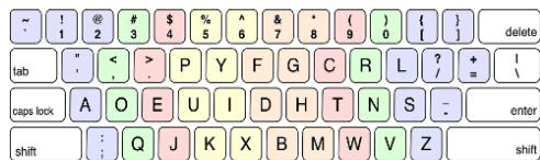
This type of keyboard layout was developed to increase the typing speed by reducing the finger movement while typing. The most frequently used letters are kept in a home row to improve typing.
