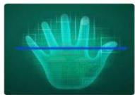
The hand of a person can also be used to verify his or her identity as every person has a unique pattern of veins in the palm, just like fingerprints. This device takes advantage of this feature; it identifies a person by scanning the palm of his hand. It uses infrared light to scan veins' patterns and blood flowing in them. Palm is even more unique than fingerprints.
