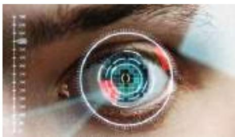
It scans the retina or iris of a person's eye to confirm the identity. This device is more secure than others as it is next to impossible to copy the retina or iris. It works by mapping the retina's blood vessel patterns of the eye. The blood vessels of retina absorb light more easily as well as can be identified with appropriate lighting.
