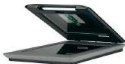
It has a glass pane and a moving optical CIS or CCD array. The light illuminates the pane, and then the image is placed on the glass pane. The light moves across the glass pane and scans the document and thus produces its digital copy. You will need a transparency adapter while scanning transparent slides.
