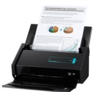
In this scanner, the document is inserted into the slot provided in the scanner. The main components of this scanner include the sheet-feeder, scanning module, and calibration sheet. The light does not move in this scanner. Instead, the document moves through the scanner. It is suitable for scanning single page documents, not for thick objects like books, magazines, etc.
