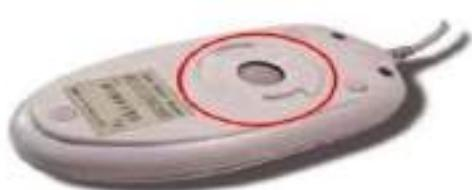
It has a system of a ball and several rollers to track its movement. It is a corded type of mouse. A mechanical mouse can be used for high performance. The drawback is that they tend to get dust into the mechanics and thus require regular cleaning.
