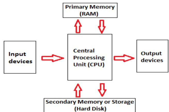
The operations of computer components are given below:
